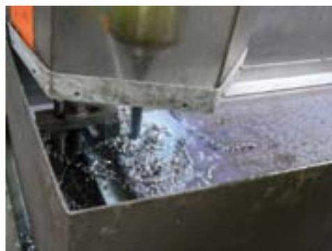
FIGURE 50 : USINAGE AVEC HUILE DE COUPE HYDROSOLUBLE
