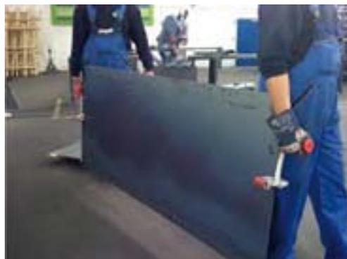
FIGURE 97 : MANUTENTION D'UNE TÔLE À L'AIDE DE PINCES MANUELLES
