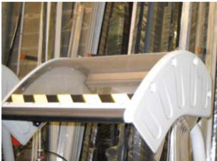
FIGURE 43 : PROTECTION DE SCIE POUR ALUMINIUM
