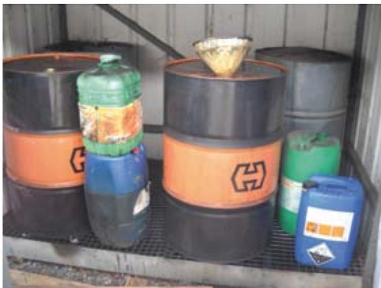
FIGURE 166 : STOCKAGE DE PRODUITS CORROSIFS AVEC D'AUTRES PRODUITS
